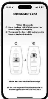
11. Within 30 seconds, press the Door UNLOCK button first, then press the Door LOCK button on the Remote Keyless Entry Fob and wait for a confirmation message.
