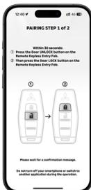
11. Within 30 seconds, press the Door UNLOCK button first, then press the Door LOCK button on the Remote Keyless Entry Fob and wait for a confirmation message.
